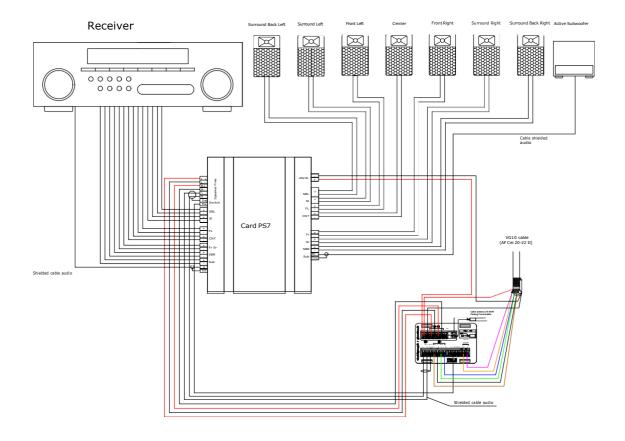
In Vivaldi systems equipped with Free, Freenet, iFree series zone control, the Giove PS7 switching board allows you to manage 7 speakers and a Subwoofer.
